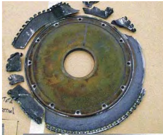
Figure 12-11. Example of ruptured compressor rotor disk
