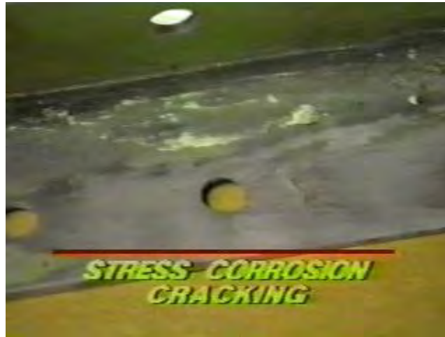
Figure 9-74. Stress Corrosion Cracking. Stress corrosion cracking may be identified by the presence of multiple, brittle appearing cracks in high-strength alloys. The crack path is often found to have followed the grain boundaries and to be branched (secondary cracks spreading sideways from the main crack). The cracks form perpendicular to the main tensile stress axis, which may be from either applied or residual stresses in the part.
