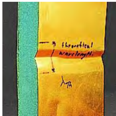
Figure 9-42. Local buckling of a face sheet into the foam core.
