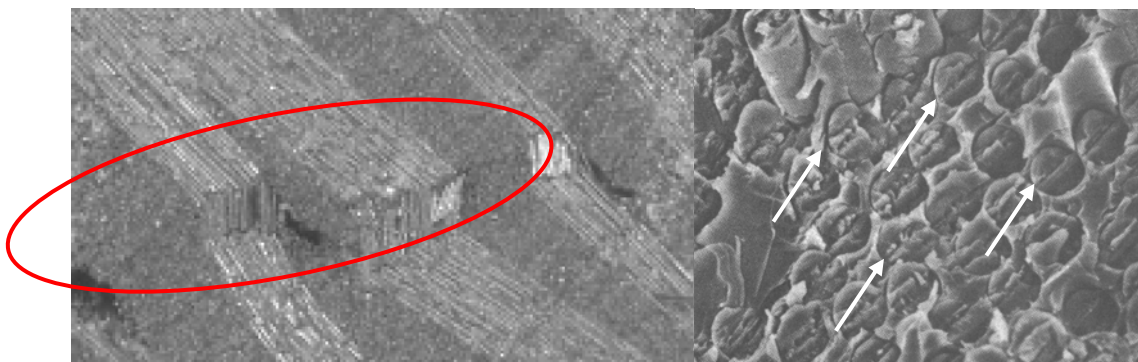
Figure 9-29. Example of fiber kinking as a result of compressive loads.
