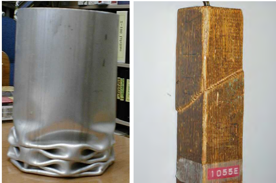
Figure 9-9. Compression (Buckling) Failure (left); Block compression failure (right)
