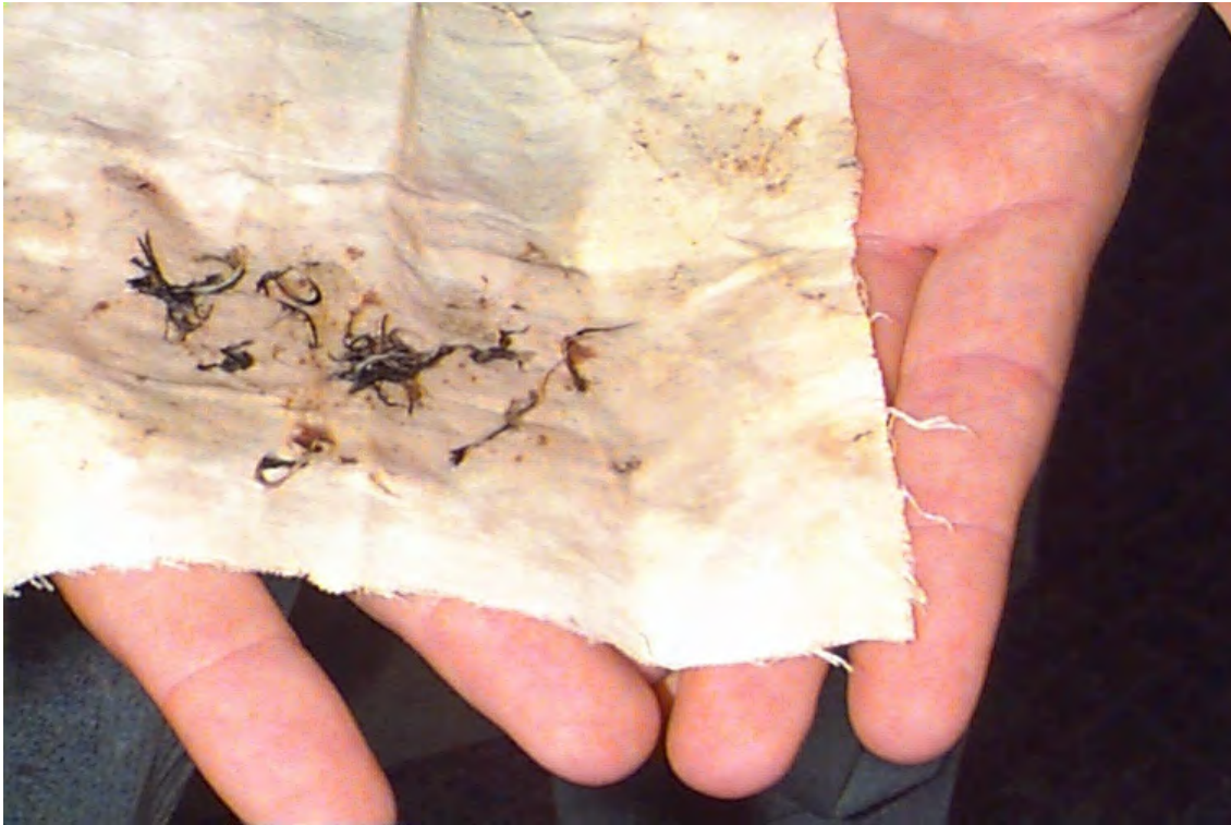
Figure 5.6.2. Bird evidence wiped from the aircraft.
