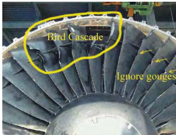
Figure 12-17. Bird ingestion damage
