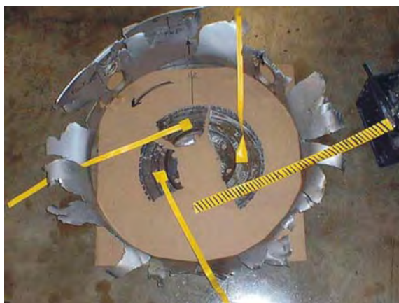
Figure 12-15. Uncontained rotor disk fragments trajectories
