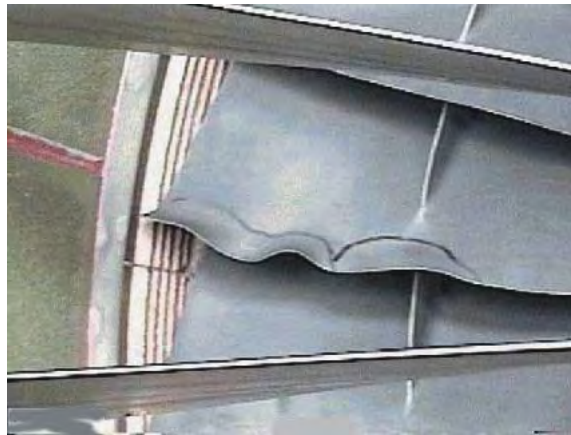
Figure 12-18. Ice ingestion ripple damage
