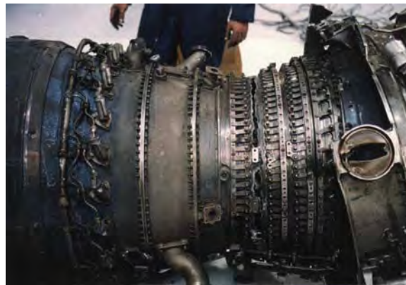
Figure 12-27. Titanium fire burn-through
