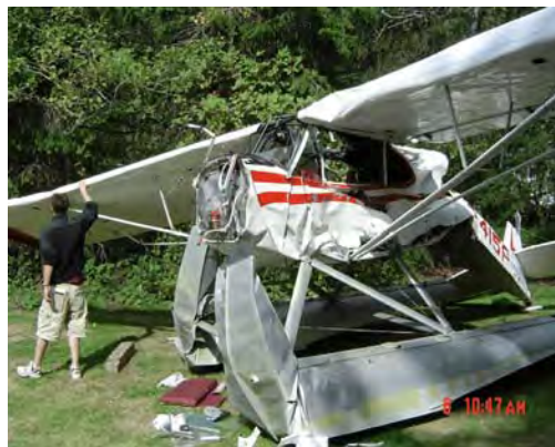
Figure 5.5.1. Water impact damage
