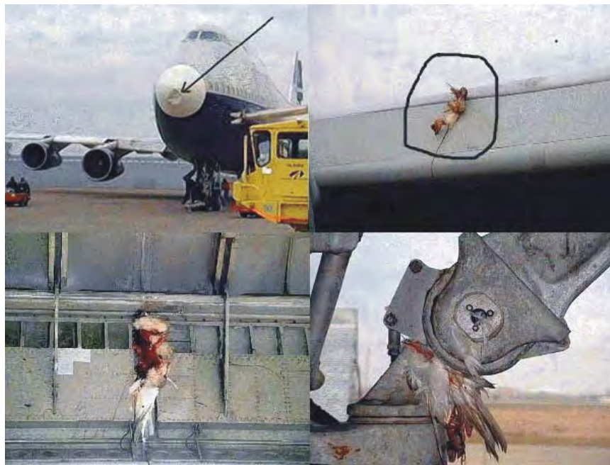
Figure 12-16. Examples of bird strike locations on aircraft
