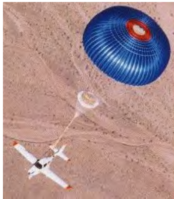
Figure 13.16.1. Rocket-deployed emergency parachute system
