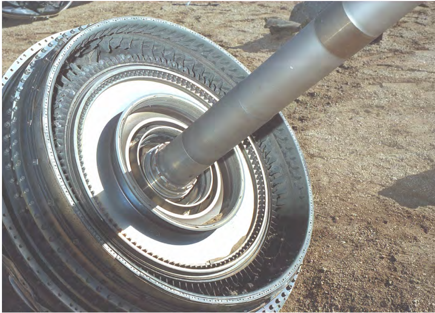
Figure 2.2 This photograph was made using a flash attachment powerful enough to illuminate the shadow areas of the photograph on a clear day under full midday sun. The damage to the engine turbine section is clearly visible.
