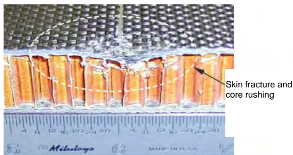
Figure 9-44 Crushed core and fractured face sheet.
