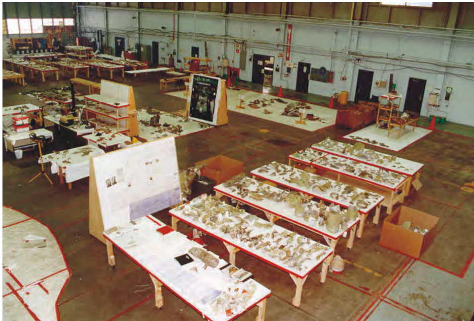
Figure 8-3. Systems Reconstruction Layout of Swissair 111 (Courtesy of Transportation safety Board of Canada)
