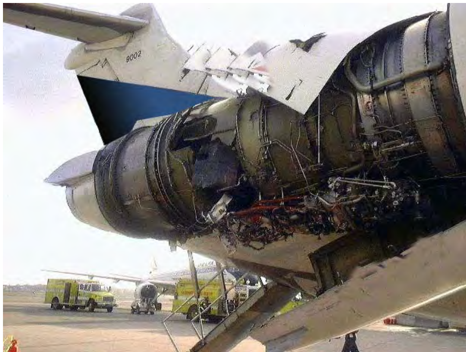
Figure 12-22. High pressure case fracture
