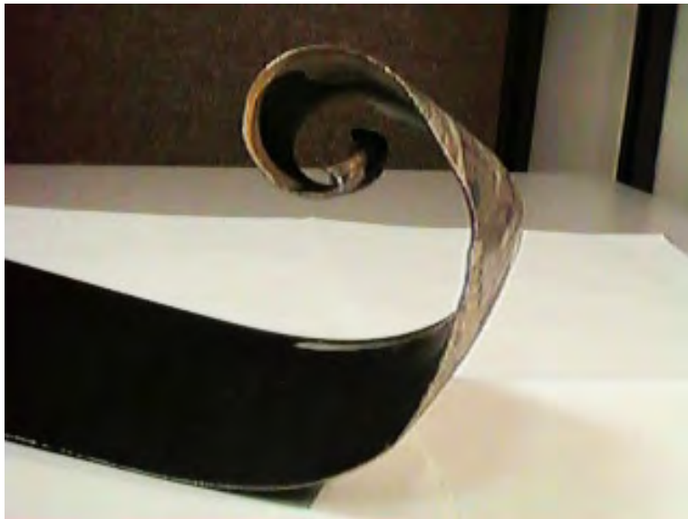
Figure 12-30. Propeller tip bent forward as a result of high RPM during a low-angle impact.
