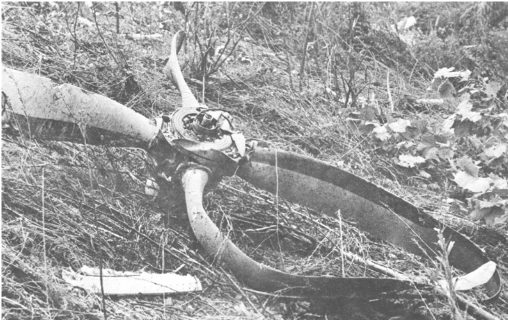
Figure 12-35. Metal Propeller under power at impact
