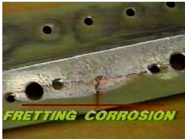
Figure 9-76. Fretting Corrosion. Fretting is identified by the appearance of surface discoloration and roughening due to the small, relative motion between two surfaces clamped together. In steels, the surface discoloration is red-brown; in aluminum fretting debris is generally a finely divided black powder.
