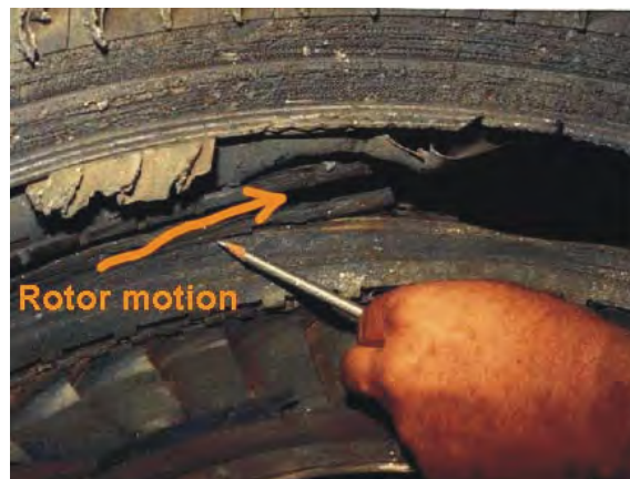
Figure 12-13. Squeeze-rupture penetration hole
