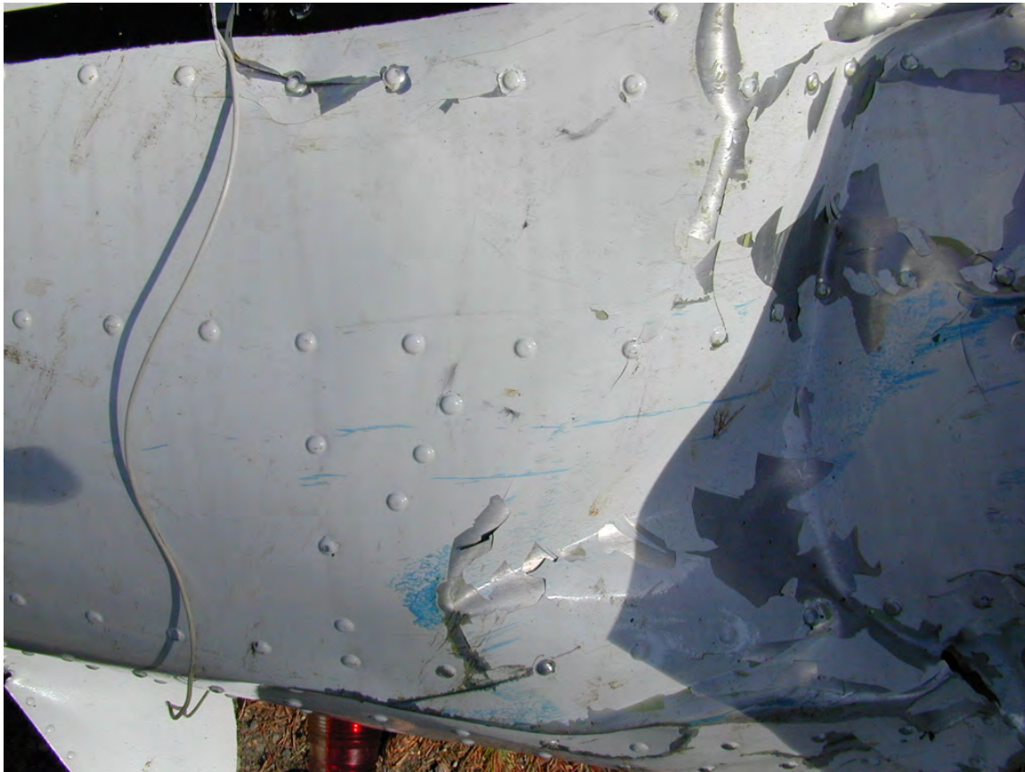
Photo 2: A vertical surface of a fuselage photographed from the side. Note the straight scratch marks and the relatively small angle formed with the longitudinal axis, showing little relative vertical movement in this collision.
