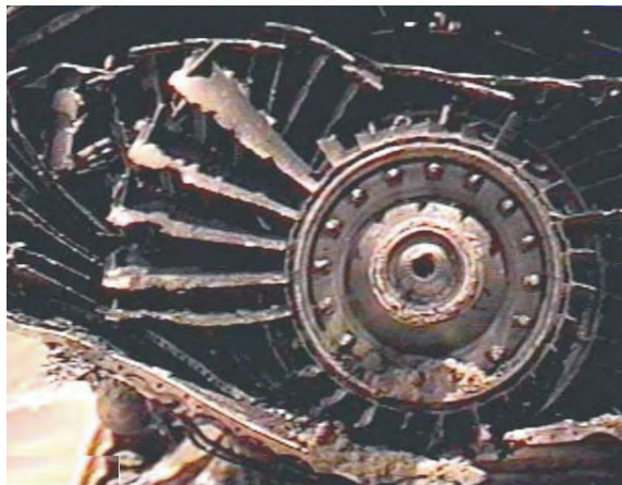
Figure 12-6. Low speed impact superimposed on high speed damage
