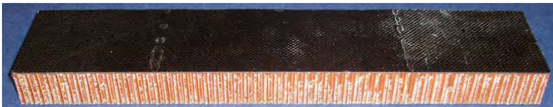
Figure 9-38. Sandwich structure with carbon fiber face sheets and a honeycomb core.
