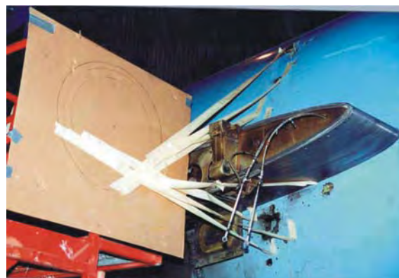
Figure 12-14. Uncontained fragments trajectory lines
