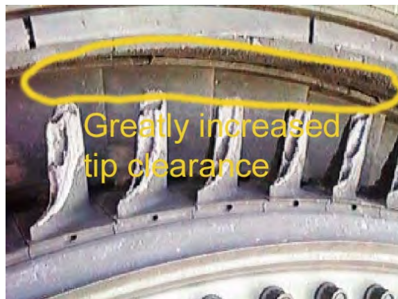
Figure 12-24. Increased tip clearance caused by overheating
