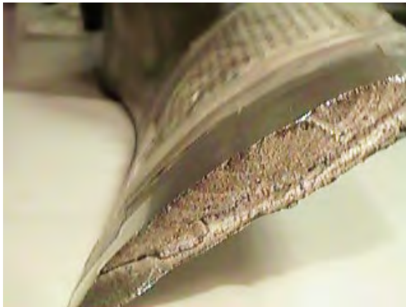
Figure 12-32. Propeller showing beach rings as a result of resonance fatigue failure
