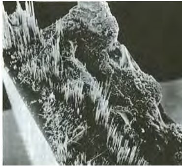
Figure 9-31. Composite specimen that failed in bending. The relatively rough area of tension failure and the relatively smooth area of compression failure are clearly identifiable.
